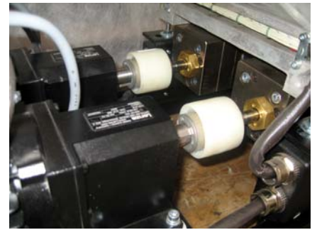
Dual pump system with separate drives
