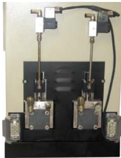
Two-pump drive and pneumatic bypass
