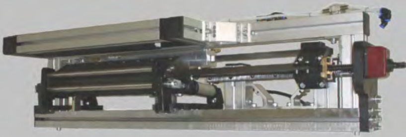
HotMelt SlotCoating Heads with Variable Coating Width
